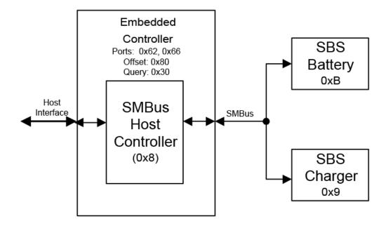
Fig. 10.2: Single Smart Battery Subsystem
