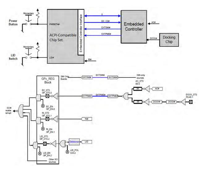
Fig. 4.13: Example of General-Purpose vs. Generic Hardware Events
