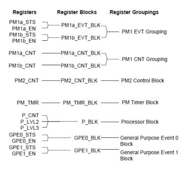
Fig. 4.6: Register Blocks versus Register Groupings
