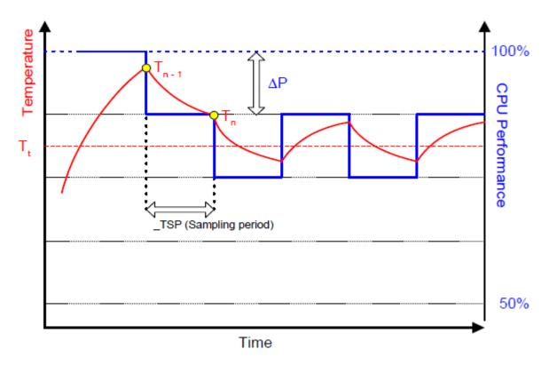
Fig. 11.3: Temperature and CPU Performance Versus Time
