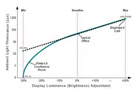
Fig. 9.2: A two-point ALS Response Curve
