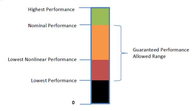
Fig. 8.10: Platform performance thresholds
