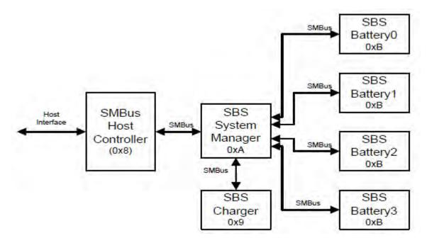
Fig. 10.1: Typical Smart Battery Subsystem (SBS)
