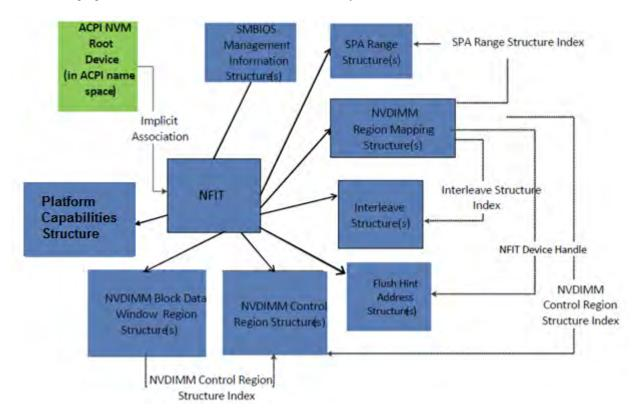
The following figure illustrates the above structures and how they are associated with each other.
