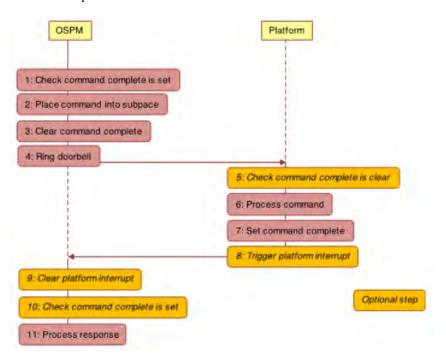
Fig. 14.1: Communication flow of the doorbell protocol
