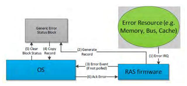
Fig. 18.1: APEI error flow example with external RAS controller
