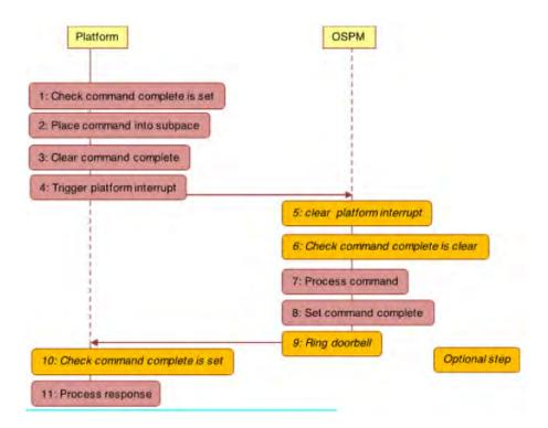
Fig. 14.2: Communication flow for notifications on slave subspaces
