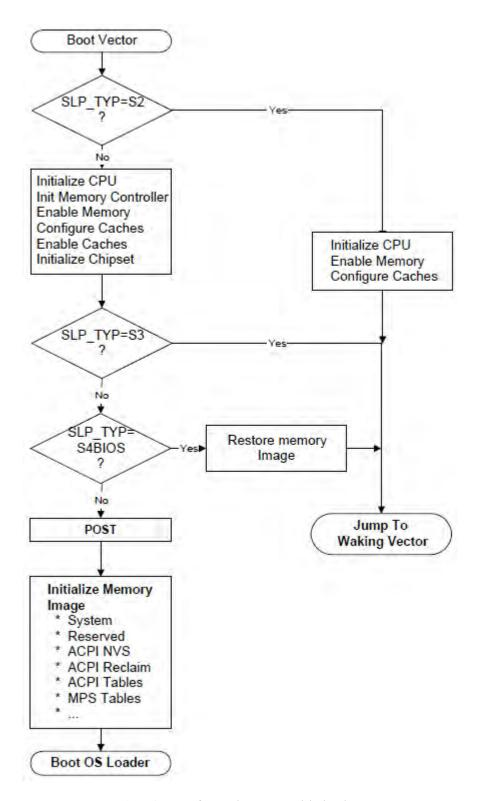
Fig. 16.2: Platform Firmware Initialization
