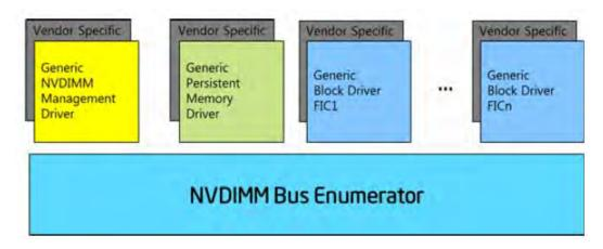
Fig. 9.8: Vendor/Device Specific Driver Loading
