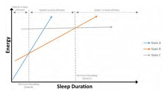
Fig. 8.9: Energy of states A,B and C versus sleep duration
