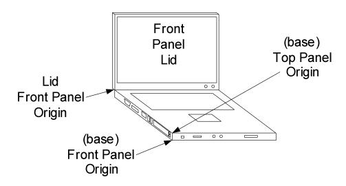
Fig. 6.2: Laptop Panel and Panel Origin Positions
