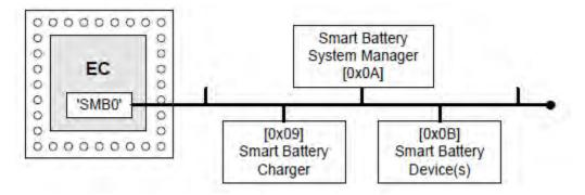
Fig. 13.2: Smart Battery Subsystem Devices
