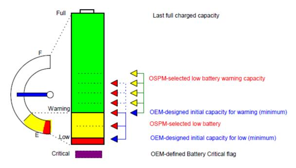
Fig. 3.6: Low Battery and Warning
