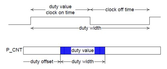
Fig. 8.2: Throttling Example
