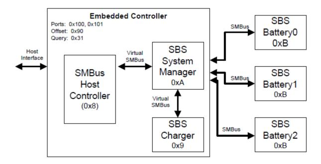
Fig. 10.3: Smart Battery Subsystem
