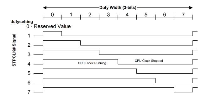
Fig. 8.4: Example Control for the STPCLK
