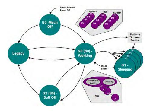
Fig. 3.1: Global System Power States and Transitions
