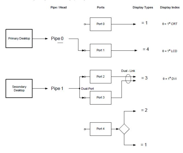
Fig. 23.1: Fig. B-1: Example Display Architecture
