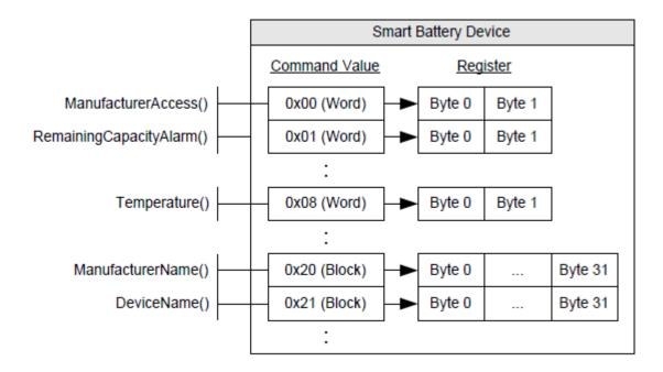
Fig. 13.3: Smart Battery Device Virtual Registers
