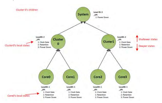
Fig. 8.7: Power states for processor hierarchy
