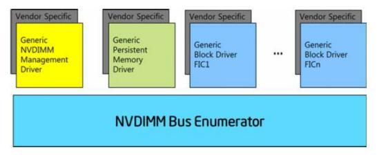
Fig. 9.8: Vendor/Device Specific Driver Loading
