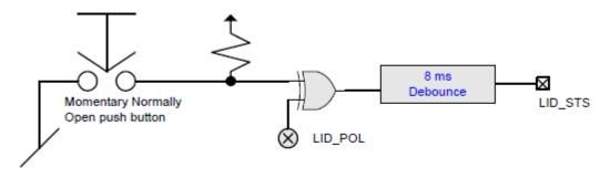
Fig. 4.14: Example Generic Address Space Lid Switch Logic
