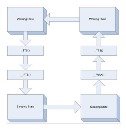
Fig. 7.1: Working / Sleeping State object evaluation flow
