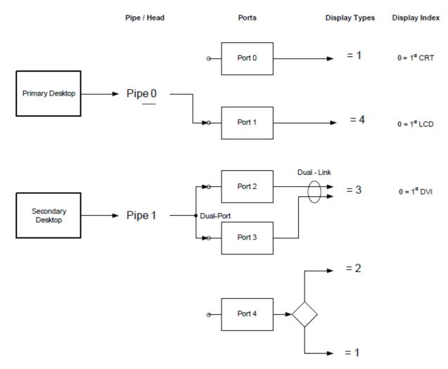
Fig. 23.1: Fig. B-1: Example Display Architecture
