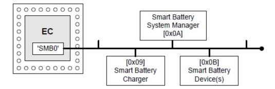
Fig. 13.2: Smart Battery Subsystem Devices
