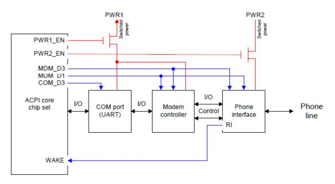
Fig. 3.2: Example Modem and COM Port Hardware
