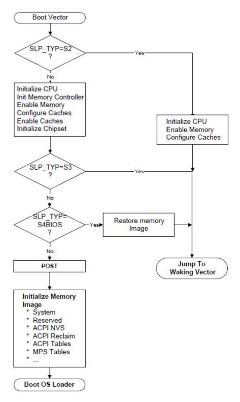
Fig. 16.2: Platform Firmware Initialization
