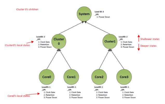
Fig. 8.7: Power states for processor hierarchy
