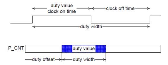
Fig. 8.2: Throttling Example
