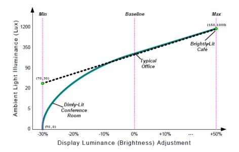
Fig. 9.2: A two-point ALS Response Curve
