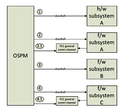
Fig. 5.11: Example: Platform with four debug triggers
