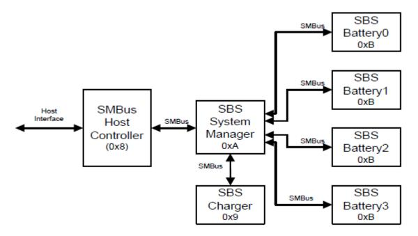
Fig. 10.1: Typical Smart Battery Subsystem (SBS)
