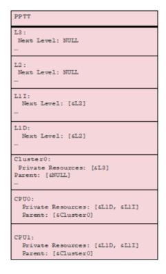
Fig. 5.13: Cache Type Structure - Type 1 Example
