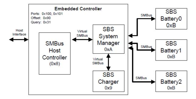
Fig. 10.3: Smart Battery Subsystem
