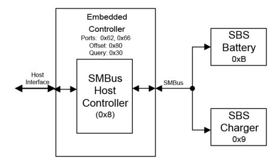
Fig. 10.2: Single Smart Battery Subsystem
