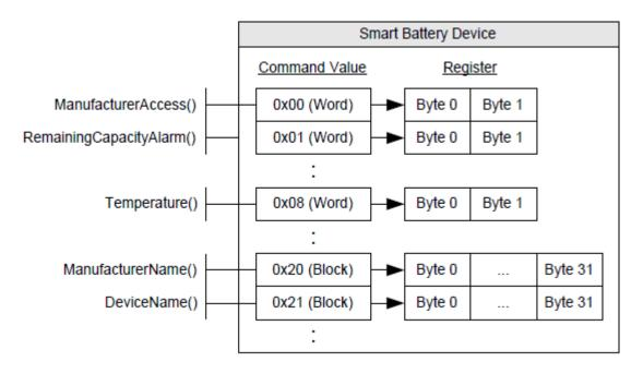
Fig. 13.3: Smart Battery Device Virtual Registers
