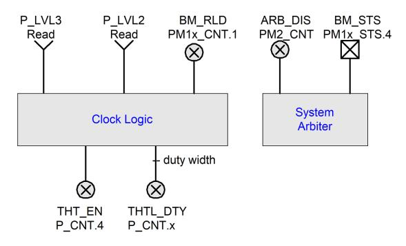
Fig. 8.5: ACPI Clock Logic (One per Processor)
