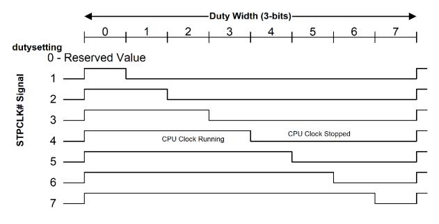
Fig. 8.4: Example Control for the STPCLK
