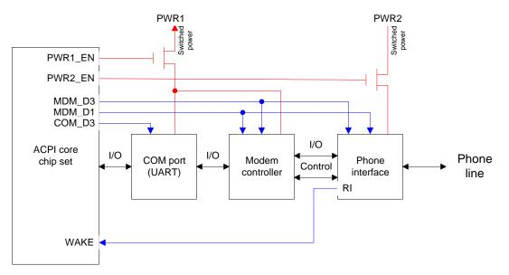
Figure 3-3 Example Modem and COM Port Hardware
