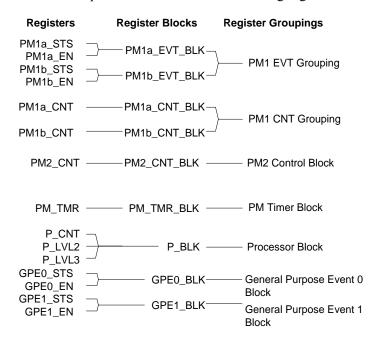
Figure 4-14 Register Blocks versus Register Groupings
