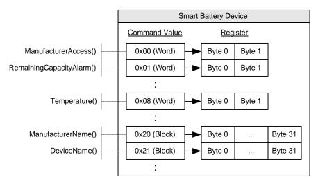
Figure 13-75 Smart Battery Device Virtual Registers
