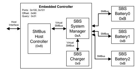
Figure 10-61 Smart Battery Subsystem
