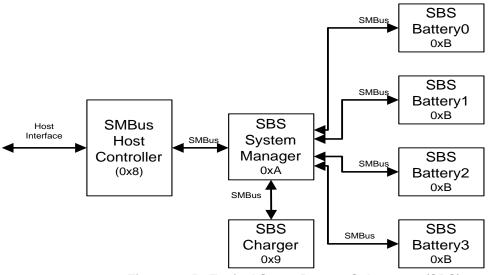
Figure 10-59 Typical Smart Battery Subsystem (SBS)
