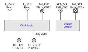
Figure 8-44 ACPI Clock Logic (One per Processor)
