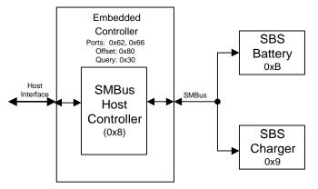
Figure 10-60 Single Smart Battery Subsystem
