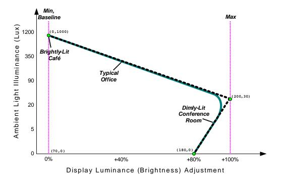
Figure 9-53 Example Response Curve for a Transflective Display
