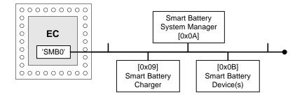
Figure 13-74 Smart Battery Subsystem Devices
