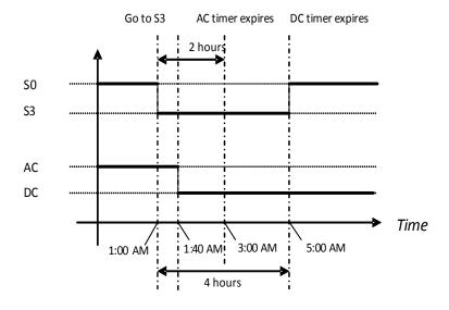
Figure 9-56 System transitions with WakeAlarm -- Timer
