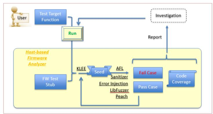
Testing UEFI firmware drivers in the developer's environment
