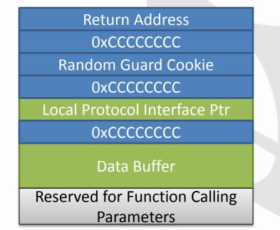
• If a buffer overflow changes the filler between locals, that overflow is detected
