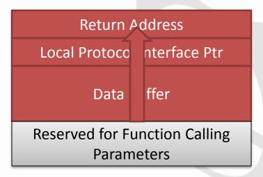
The MSVC /GS compiler switch inserts a randomized guard cookie onto the stack between the return address and locals
