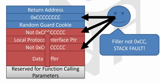
However, 0xCC is easy to forge, and the check comes just before return, not immediately after the buffer overflow
