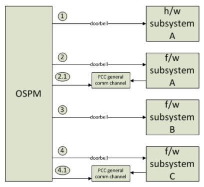
Figure 5-25 Example: Platform with 4 debug triggers
