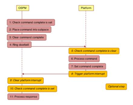
Figure 14-72 Communication flow of the doorbell protocol
