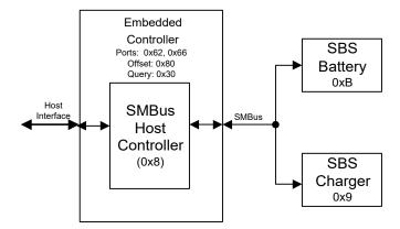
Figure 10-56 Single Smart Battery Subsystem
