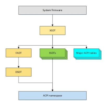
System firmware updates the ACPI tables as necessary with information only available at runtime before handing off control to the boostrap loader.
