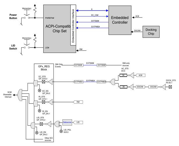
Figure 4-13 Example of General-Purpose vs. Generic Hardware Events
