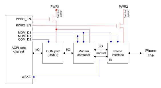
Figure 3-2 Example Modem and COM Port Hardware
