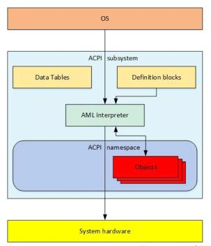
The ACPI subsystem consists of two types of data structures: data tables and definition blocks.
