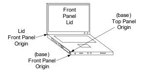
Figure 6-30 Laptop Panel and Panel Origin Positions
