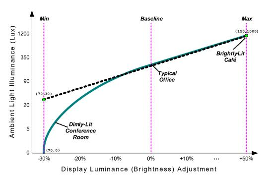
Figure 9-48 A two-point ALS Response Curve
