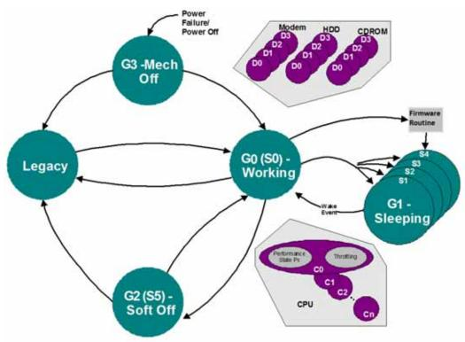
Figure 3-1Global System Power States and Transitions
