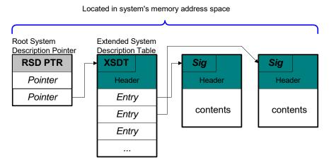
Figure 5-15 Root System Description Pointer and Table
