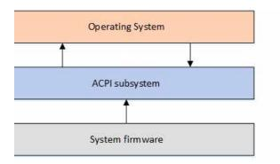
The ACPI subsystem is an interface layer between the System firmware and the OS. The arrows indicate data flow.
