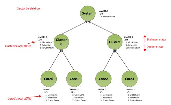
Figure 8-42 Power states for processor hierarchy
