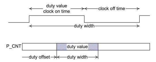
Figure 8-37 Throttling Example
