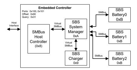
Figure 10-57 Smart Battery Subsystem
