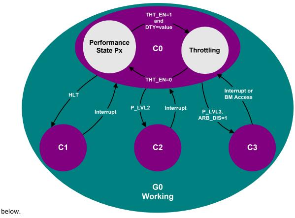
states (P-states). A diagram of processor power states is provided
