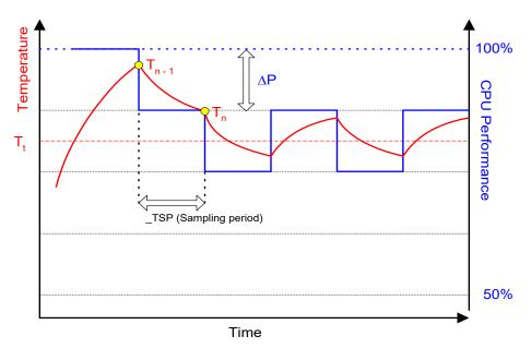
Figure 11-63 Temperature and CPU Performance Versus Time
