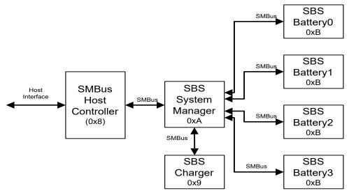
Figure 10-55 Typical Smart Battery Subsystem (SBS)
