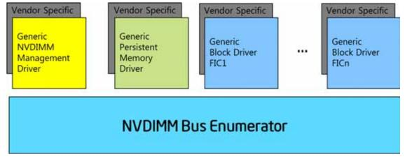
Figure 9-54 Vendor/Device Specific Driver Loading
