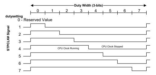
Figure 8-39 Example Control for the STPCLK#
