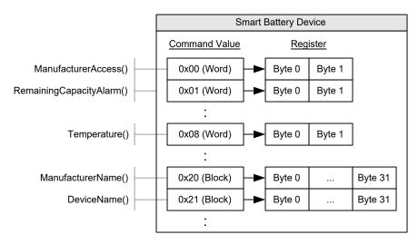
Figure 13-71 Smart Battery Device Virtual Registers
