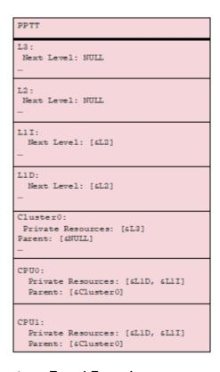
Figure 5-26 Cache Type Structure - Type 1 Example
