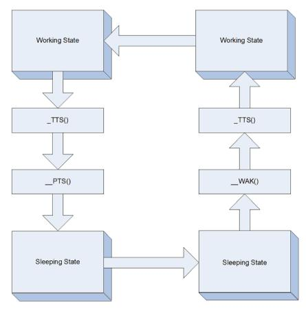
Figure 7-35 Working / Sleeping State object evaluation flow
