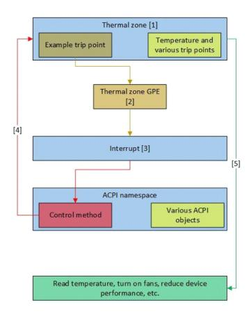
When the system initially finds a thermal zone [1] in the namespace, it loads the thermal zone handler to evaluate the thermal zone to determine the temperature and trip points.
