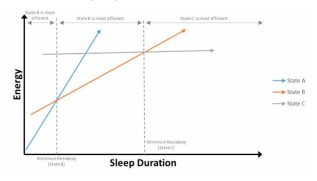
Figure 8-44 Energy of states A,B and C versus sleep duration
