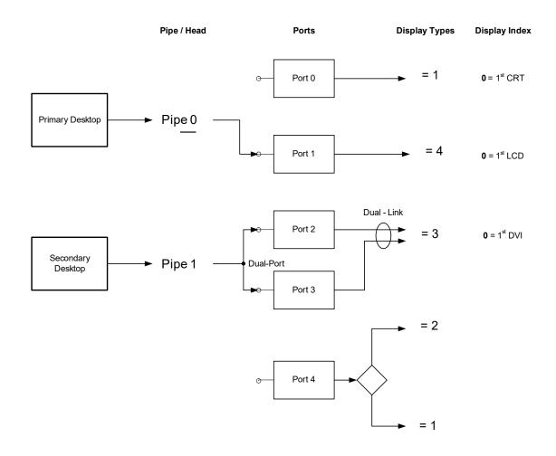
Figure B-1 Example Display Architecture
