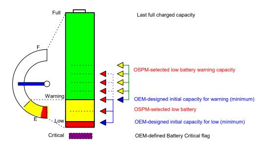
Figure 3-4 Low Battery and Warning
