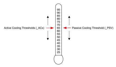
Figure 11-64 Active and Passive Threshold Values
