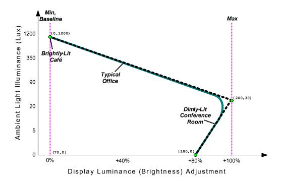
Figure 9-49 Example Response Curve for a Transflective Display
