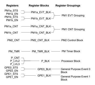
Figure 4-6 Register Blocks versus Register Groupings
