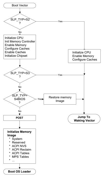
Figure 16-75 Platform Firmware Initialization
