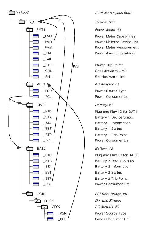
Figure 10-60 Power Meter and Power Source/Docking Namespace Example
