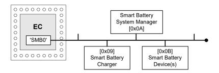
Figure 13-70 Smart Battery Subsystem Devices
